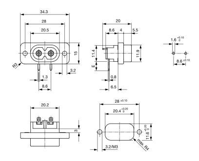
$$\begin{split} E &= PCB \ terminal \ standard \ (additional \ solder): 6.9 \ mm \\ E &= PCB \ terminal \ short \ (additional \ solder): 0.6 \ mm \end{split}$$
