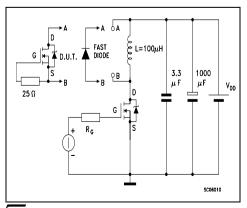
Figure 19: Unclamped Inductive Wafeform
