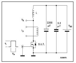
Figure 17: Switching Times Test Circuit For Resistive Load
