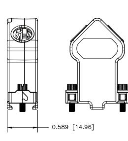
PLATING: **NICKEL OVER COPPER** STEEL, ZINC PLATED JACKSCREWS: **HOUSING SCREWS:** STEEL, ZINC PLATED STEEL, ZINC PLATED STRAIN RELIEF SCREWS: **COVER PLATE:** STEEL, ZINC PLATED STRAIN RELIEF CLAMP: STEEL. ZINC PLATED
