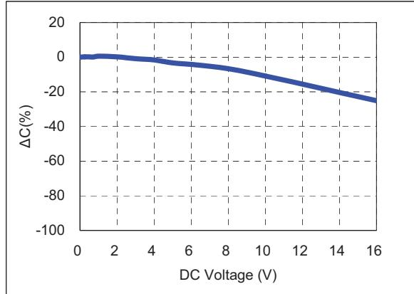
4) Bias TCC characteristics (Agilent 4284A, 1kHz, 1Vrms, 8Vdc)
