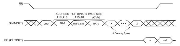
Figure 18-2. Main Memory Page to Buffer Transfer (Data from Flash Page Read into Buffer)
