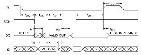
Figure 17-3. Waveform  $3 - \text{RapidS Mode } 0 \text{ (}F_{\text{MAX}} = 66\text{MHz}\text{)}$
