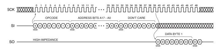
Figure 19-3. Continuous Array Read (Low Frequency: Opcode 03H)
