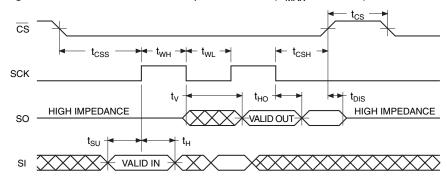
Figure 17-4. Waveform 4 – RapidS Mode 3 ( $F_{MAX}$  = 66MHz)
