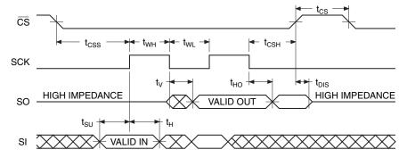
Figure 17-2. Waveform 2 – SPI Mode 3 Compatible (for Frequencies up to 66MHz)
