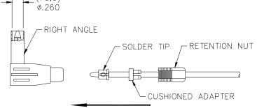
6. ASSEMBLE SOLDER TIP AND CUSHIONED ADAPTER. ALINE THE BANANA PLUG THRU HOLE TO SOLDER TIP. THREAD BY SLIDING SOLDER TIP ASSEMBLY INTO BANANA PLUG THRU HOLE AND TIGHTEN RETENTION NUT TO RIGHT ANGLE.
