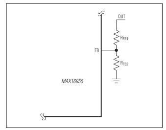
Figure 2. Adjustable Output Voltage
