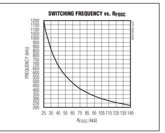
Figure 3. Switching Frequency vs. RFOSC
