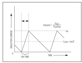
Figure 1. Pulse-Skipping/Discontinuous Crossover Point
