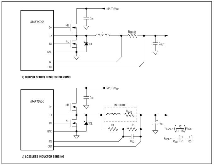
Figure 4. Current-Sense Configurations
