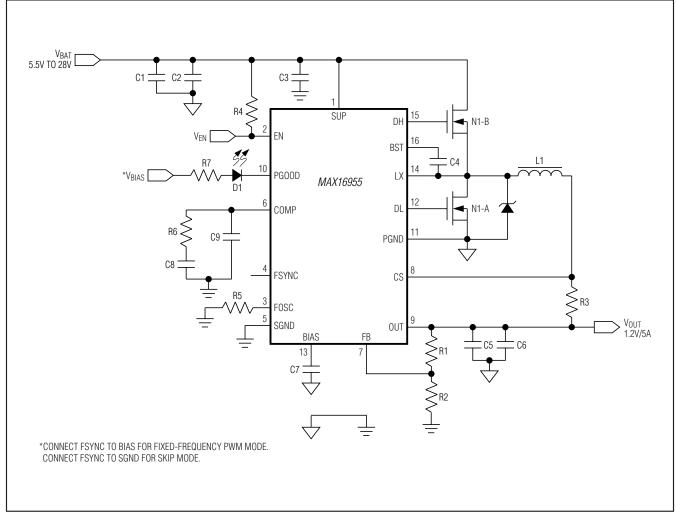
Figure 7. Typical Operating Circuit for Adjustable Output Voltage, V<sub>OUT</sub> = 1.2V/5A
