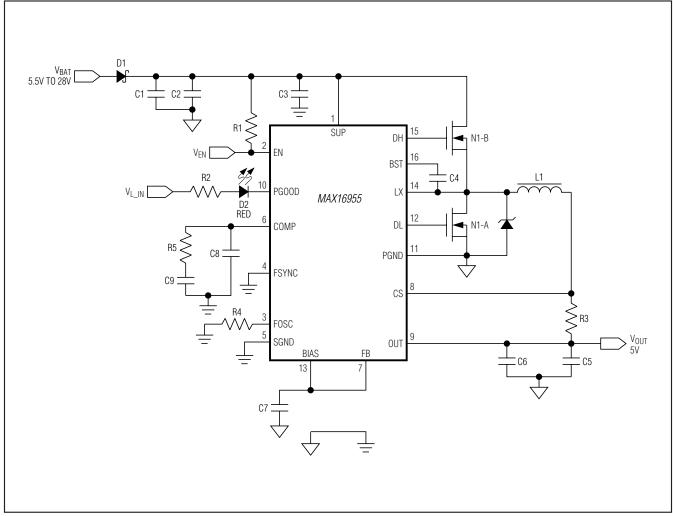
Figure 6. Typical Operating Circuit for  $V_{OUT} = 5V$
