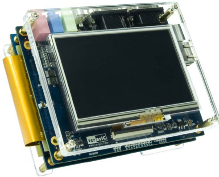
Figure 1.1. The BRICK form of combining the MTDB to an Altera Cyclone III Starter Board.
