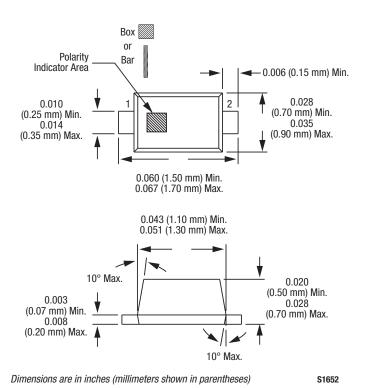
Figure 5. SC-79 Package Dimension Drawing
