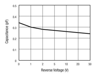
Figure 3. Capacitance vs Reverse Voltage (1 MHz to 1 GHz)
