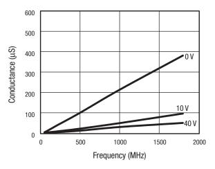
Figure 4. Conductance vs Frequency and Reverse Voltage
