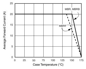
Figure 1. Forward Derating Curve (Total)
