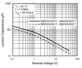
Figure 5. Typical Junction Capacitance Per Diode
