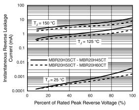
Figure 4. Typical Reverse Characteristics Per Diode
