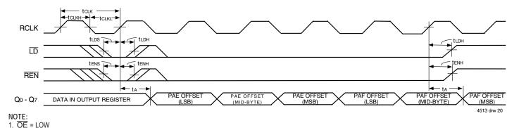
Figure 17. Parallel Read of Programmable Flag Registers (IDT Standard and FWFT Modes) for the IDT72V291
