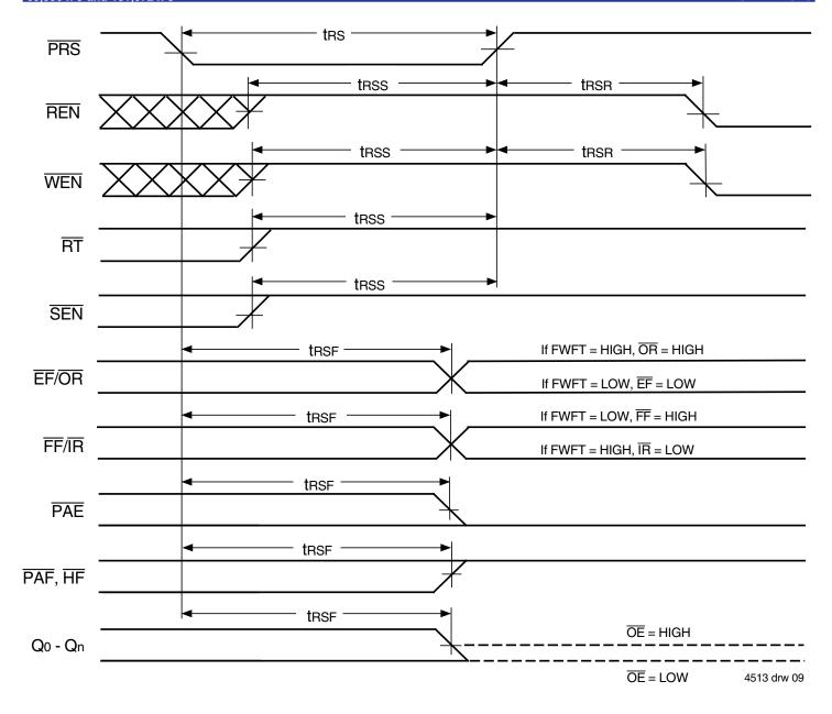
Figure 6. Partial Reset Timing
