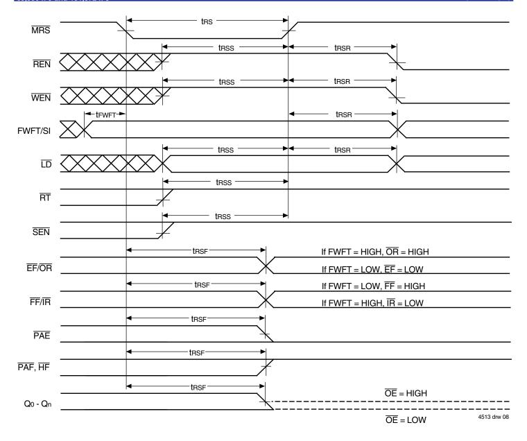
Figure 5. Master Reset Timing
