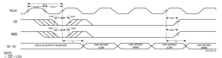
Figure 16. Parallel Read of Programmable Flag Registers (IDT Standard and FWFT Modes) for the IDT72V281
