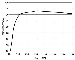
FIGURE 6. BOOST PWM EFFICIENCY vs LOAD
