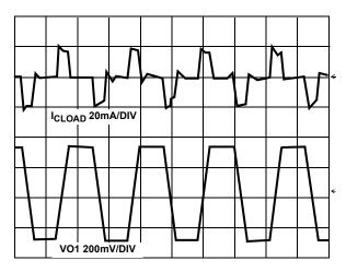
FIGURE 13. ZERO LOAD 22kHz TONE AT CATHODE OF DIODE AND DRIVING CURRENT CHARGING AND DISCHARGING CLOAD
