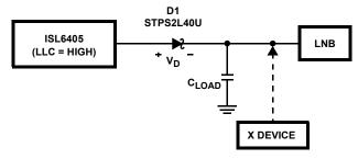
FIGURE 11. DC BACK-BIAS PROTECTION CIRCUIT
