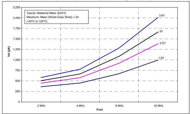
FIGURE 26-23: PIC16F707 TYPICAL IDD vs. FOSC OVER VDD, INTOSC MODE, VCAP = 0.1µF
