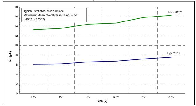
FIGURE 26-48: PIC16LF707 WDT IPD vs. VDD
