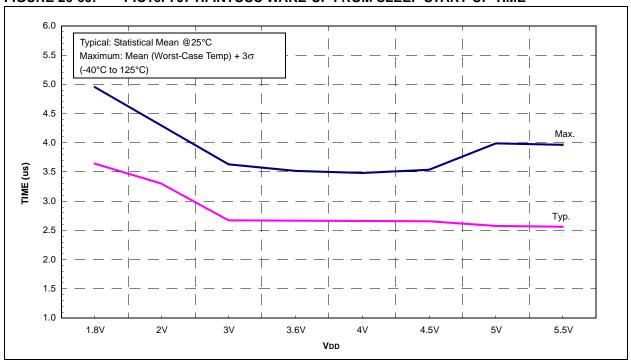
FIGURE 26-61: PIC16F707 A/D INTERNAL RC OSCILLATOR PERIOD
