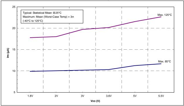
FIGURE 26-46: PIC16LF707 ADC IPD vs. VDD
