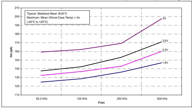
FIGURE 26-20: PIC16LF707 MAXIMUM IDD vs. Fosc OVER VDD, INTOSC MODE
