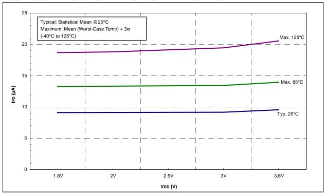
FIGURE 26-33: PIC16F707 BOR IPD vs. VDD, VCAP =  $0.1\mu$ F
