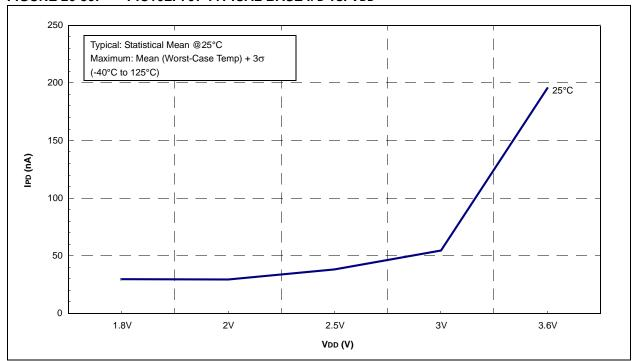
FIGURE 26-31: PIC16F707 FIXED VOLTAGE REFERENCE IPD vs. VDD, VCAP = 0.1 µF
