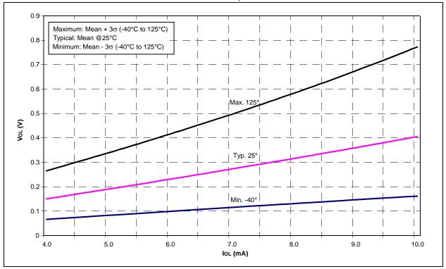
FIGURE 26-57: Vol vs. Iol OVER TEMPERATURE, VDD = 1.8V
