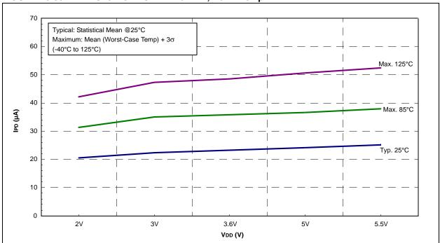
FIGURE 26-34: PIC16LF707 BOR IPD vs. VDD
