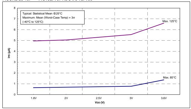
FIGURE 26-47: PIC16F707 WDT IPD vs. VDD, VCAP =  $0.1\mu$ F
