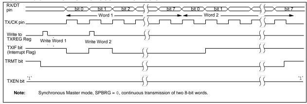
FIGURE 18-7: SYNCHRONOUS TRANSMISSION (THROUGH TXEN)
