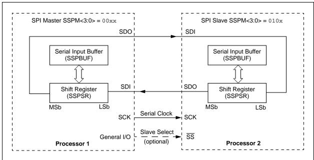
FIGURE 19-2: SPI MODE BLOCK DIAGRAM
