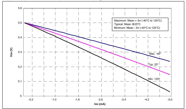
FIGURE 26-53: Voh vs. Ioh OVER TEMPERATURE, VDD = 3.6V
