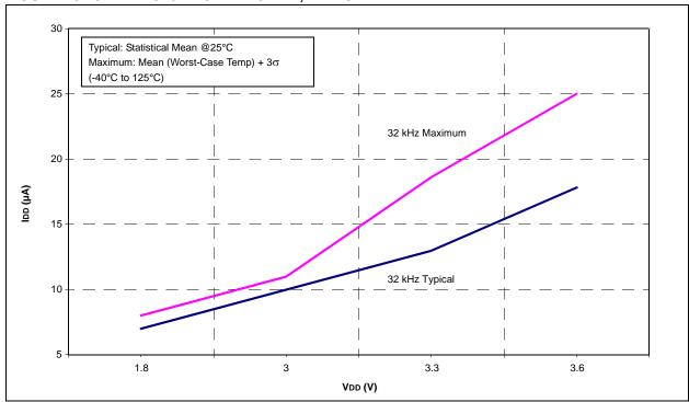
FIGURE 26-19: PIC16F707 MAXIMUM IDD vs. FOSC OVER VDD, INTOSC MODE, VCAP = 0.1µF
