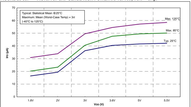
FIGURE 26-36: PIC16LF707 CAP SENSE HIGH POWER IPD vs. VDD
