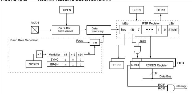
FIGURE 18-2: AUSART RECEIVE BLOCK DIAGRAM
