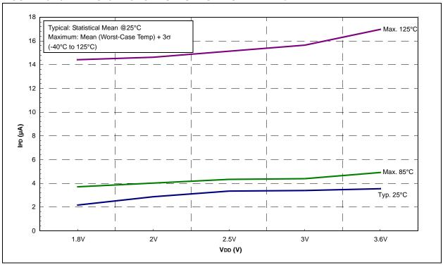
FIGURE 26-41: PIC16F707 T1OSC 32 kHz IPD vs. VDD, VCAP = 0.1μF
