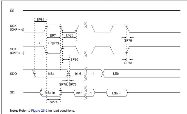
FIGURE 25-18: SPI SLAVE MODE TIMING (CKE = 0)
