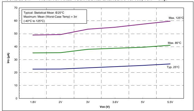
FIGURE 26-32: PIC16LF707 FIXED VOLTAGE REFERENCE IPD vs. VDD
