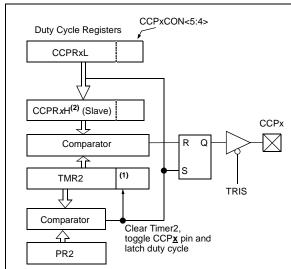
Note 1: The 8-bit timer TMR2 register is concatenated with the 2-bit internal system clock (Fosc), or 2 bits of the prescaler, to create the 10-bit time base.
