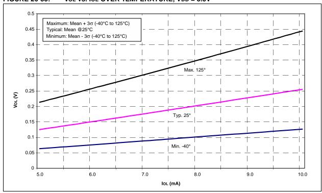
FIGURE 26-56: Vol vs. Iol OVER TEMPERATURE, VDD = 3.6
