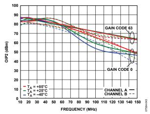
Figure 20. OIP2 vs. Frequency at Gain Code 0 and Gain Code 63, 2 V p-p Composite Output
