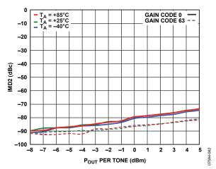
Figure 27. IMD2 vs. Output Power (Pour) at Minimum and Maximum Gain Codes, 10 MHz Frequency
