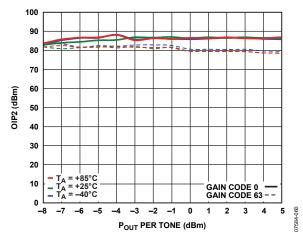
Figure 24. OIP2 vs. Output Power (Ρουτ) at Minimum and Maximum Gain Codes, 10 MHz Frequency
