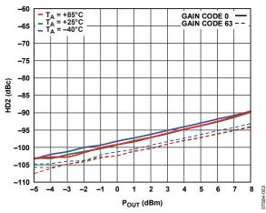
Figure 25. HD2 vs. Output Power (Pour) at Gain Code 0 and Gain Code 63, 10 MHz Frequency
