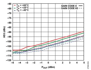
Figure 28. HD3 vs. Output Power (Pour) for Gain Code 0 and Gain Code 63, 10 MHz Frequency
