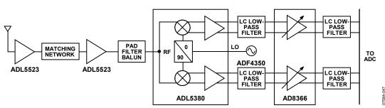
Figure 51. Direct Conversion Receiver Block Diagram
