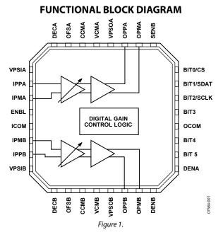
The output common-mode voltage defaults to  $V_{POS}/2$  but can be programmed via the VCMA and VCMB pins over a range of voltages. The input common-mode voltage also defaults to  $V_{POS}/2$  but can be driven down to 1.5 V. A built-in, dc offset compensation loop can be used to eliminate dc offsets from prior stages in the signal chain. This loop can also be disabled if dccoupled operation is desired.
