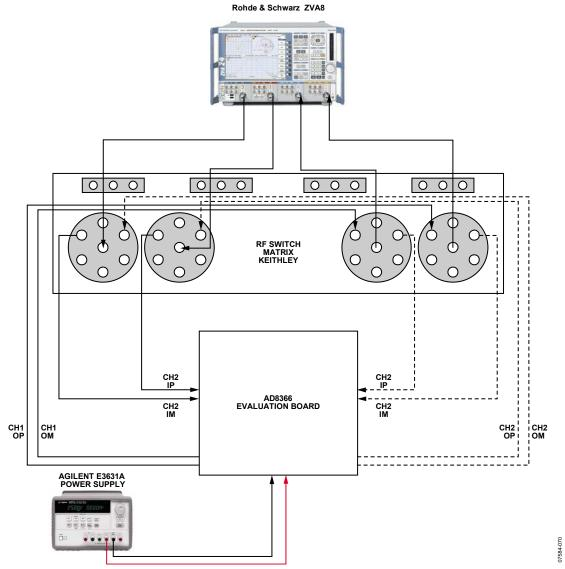
Figure 59. Characterization Setup, Differential Measurements
