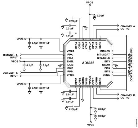
Figure 50. Basic Connections
