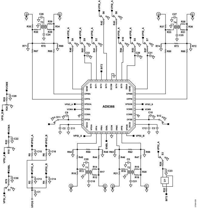
Figure 60. Evaluation Board Schematic
