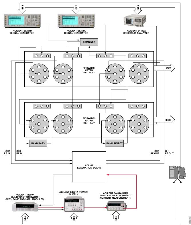
Figure 58. Characterization Setup, Single-Ended Measurements
