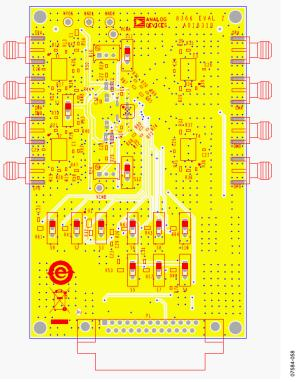
Figure 62. AD8366 Evaluation Board PCB, Bottom Side
