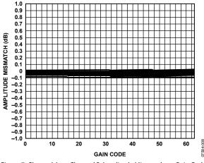
Figure 7. Channel A-to-Channel B Amplitude Mismatch vs. Gain Code, 2 V p-p Output
