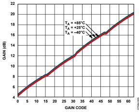
Figure 5. Gain vs. Gain Code at 500 kHz, 3 MHz, 10 MHz, and 50 MHz
