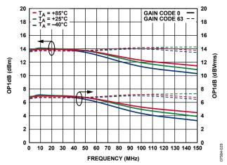
*Figure 14. OP1dB vs. Frequency at Gain Code 0 and Gain Code 63*
