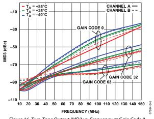
Figure 16. Two-Tone Output IMD3 vs. Frequency at Gain Code 0, Gain Code 32, and Gain Code 63, 2 V p-p Composite Output
