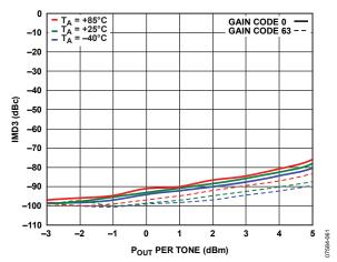
Figure 26. IMD3 vs. Output Power (Pour) at Minimum-to-Maximum Gain Codes, 10 MHz Frequency
