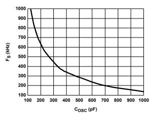
FIGURE 10. SWITCHING FREQUENCY vs COSC
