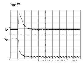
FIGURE 20. SHORT-CIRCUIT PROTECTION
