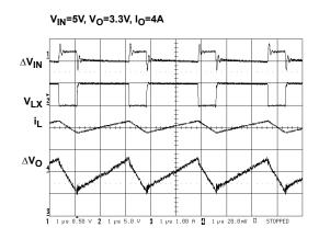
FIGURE 14. SWITCHING WAVEFORMS
