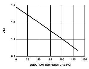
FIGURE 12. VTJ vs JUNCTION TEMPERATURE
