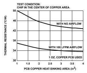
FIGURE 7. EL7564CM  $\theta_{\mbox{\scriptsize JA}}$  vs COPPER AREA
