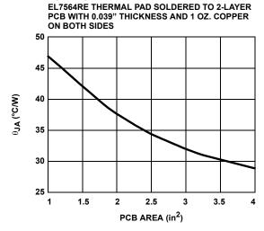
FIGURE 8. EL7564CRE THERMAL RESISTANCE vs PCB AREA - NO AIRFLOW
