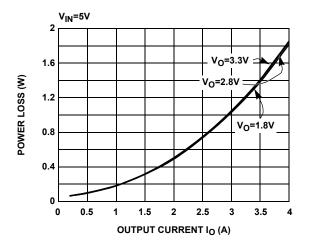
FIGURE 3. EL7564CM TOTAL CONVERTER POWER LOSS
