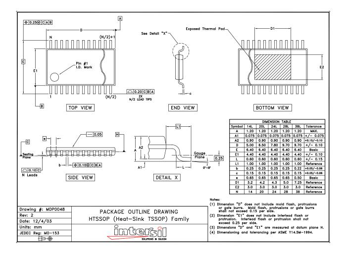
NOTE: The package drawing shown here may not be the latest version. To check the latest revision, please refer to the Intersil website at <a href="http://www.intersil.com/design/packages/index.asp">http://www.intersil.com/design/packages/index.asp</a>
