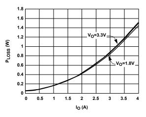
FIGURE 4. EL7564CRE TOTAL CONVERTER POWER LOSS
