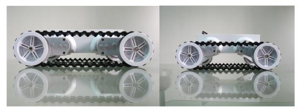
Each gearbox has an 87:1 ratio includes an optical quadrature encoder that gives 1000 pulses over 3 revolutions of the output shaft. The chassis can be upgraded to include four motors and encoders making it ideal for mecanum wheels.
