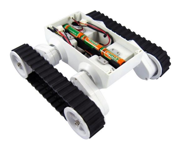
Rover 5 is a new breed of tracked robot chassis designed specifically for students and hobbyist. Unlike conventional tracked chassis's the clearance can be adjusted by rotating the gearboxes in 5-degree increments. "Stretchy" rubber treads maintain tension as the clearance is raised.
