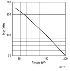
Figure 3. f<sub>OSC</sub> vs OSC Capacitor Values
