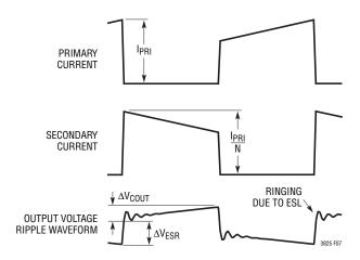
Figure 7. Typical Flyback Converter Waveforms
