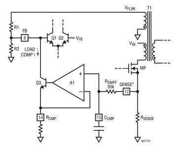
Figure 1. Load Compensation Diagram
