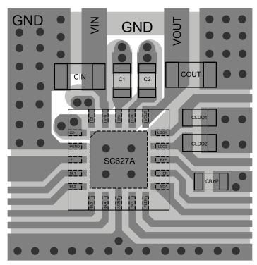
Figure 1 — Recommended PCB Layout
