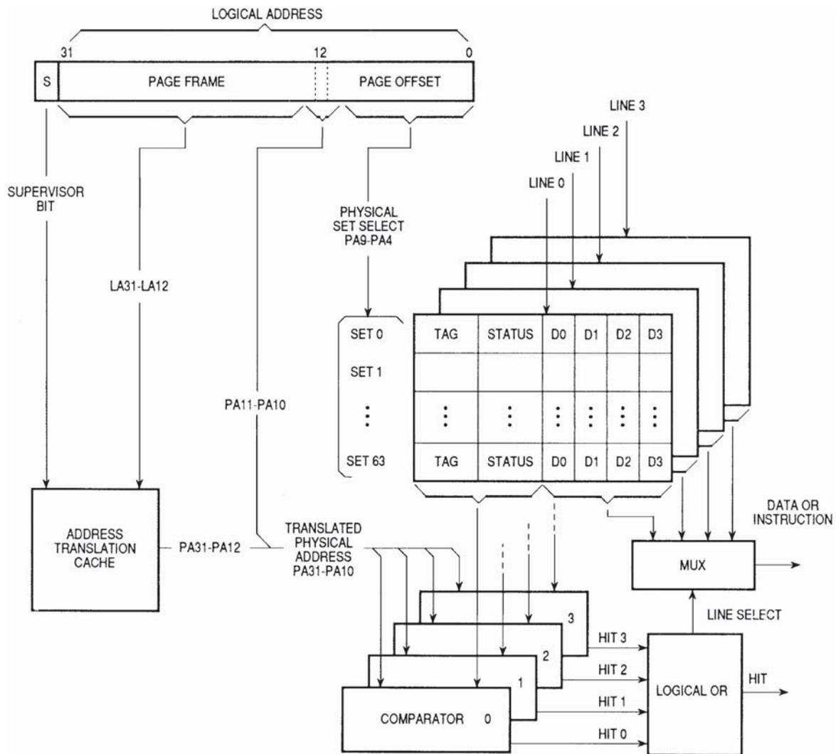
The caches are accessed by physical addresses from the on-chip MMUs. The translation of the upper bits of the logical address occurs concurrently with the accesses into the set array in the cache by the lower address bits. The output of the ATC is compared with the tag field in the cache to determine if one of the lines in the selected set matches the translated physical address. If the tag matches and the entry is valid, then the cache has a hit.
