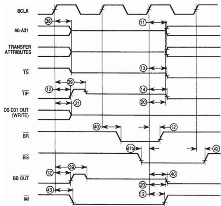
Figure 13. Snoop Hit Timing
