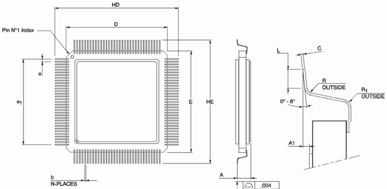
\* Reduce pin count shown for clarity, 49 pins per side
