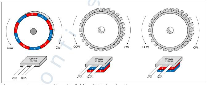
Figure 1 Sensor Assembly and Definition of Rotating Directions
