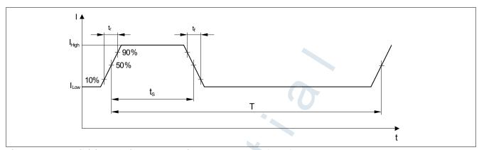
Figure 8 Definition of Rise and Fall time; Duty Cycle=  $(t_s / T) \times 100\%$
