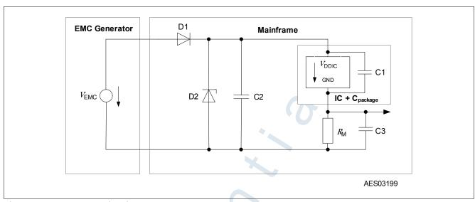
Figure 9 EMC test circuit
