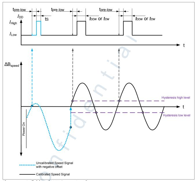
Figure 7 **Definition of PWM Current Interface**
