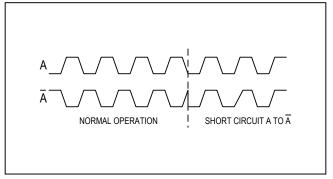
Figure 4. Short-Circuit Detection
