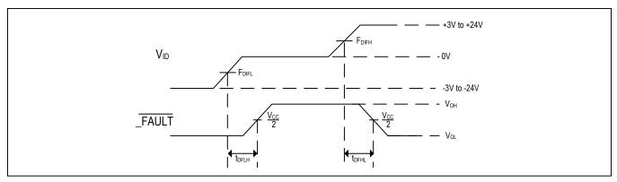
Figure 3. Fault Detection Timing
