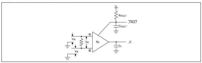
Figure 1. Receiver Test Circuit
