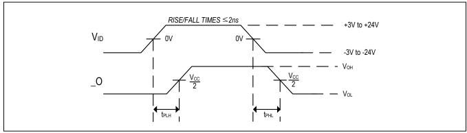
Figure 2. Receiver Propagation Delay
