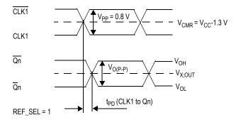
Figure 7. MC100ES8111 AC Reference Measurement Waveform (PECL Input)
