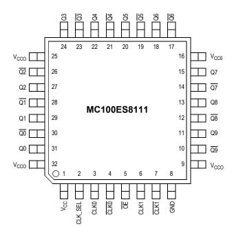
Figure 1. MC100ES8111 Logic Diagram
