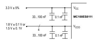
Figure 4. V<sub>CC</sub>, V<sub>CCO</sub> Power Supply Bypass
