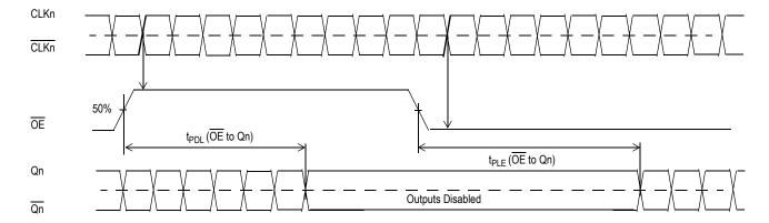
Figure 5. MC100ES8111 Output Disable/Enable Timing
