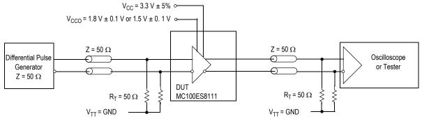
Figure 3. MC100ES8111 AC Test Reference
