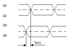
Figure 8. Output-to-Output Skew
